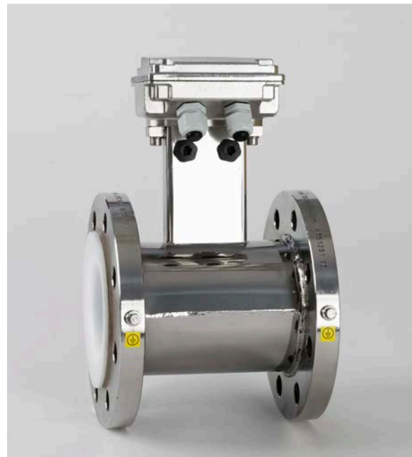
The MS2500 shown with stainless steel body, PTFE liner and junction box for remote mounted converter.
